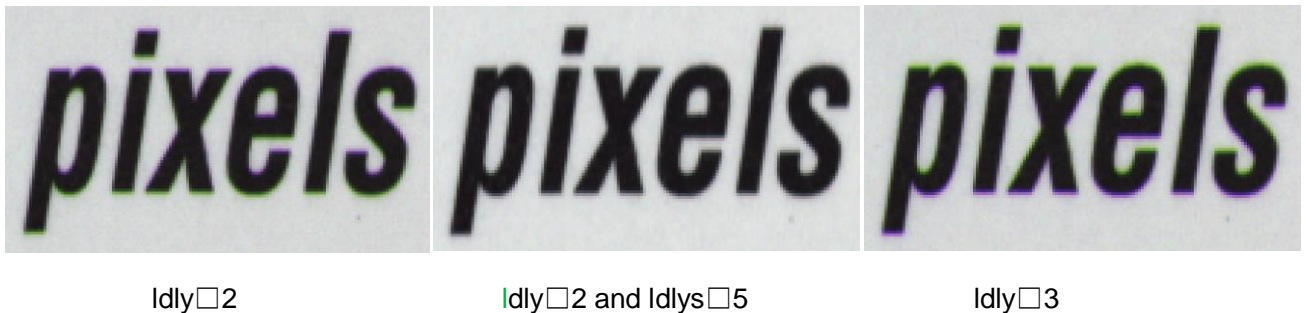
Figure 4-15-1 Line Fine Adjusting Correction
