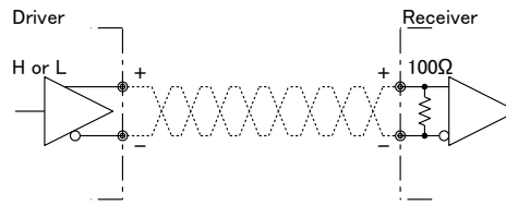
Figure 3-3-2 Circuit of LVDS
