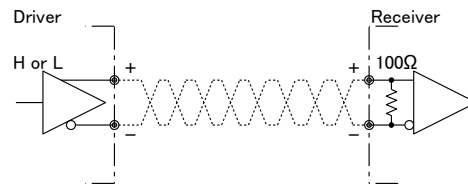
Figure 3-3-2 Circuit of LVDS
