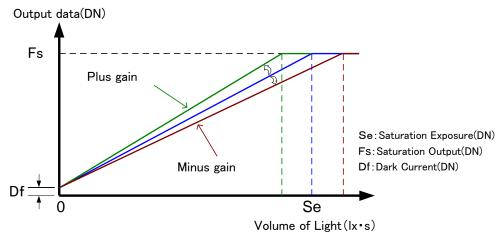
Figure 4-8-1 Gain Adjustment
