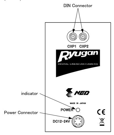
Figure 3-2-1 Input / Output Connectors and Power connector
