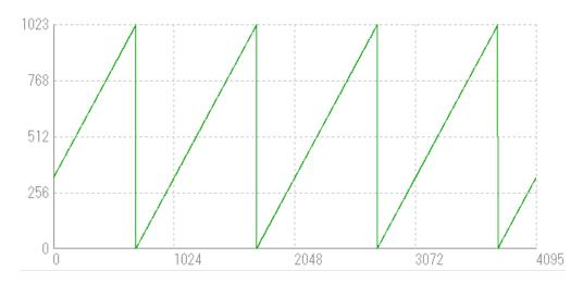
Figure 4-10-4-7 Waveforms of the XY(horizontal vertical) ramp pattern on Mono10
