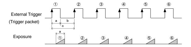
Figure 4-7-3-1 External Trigger (TriggerWidth) Exposure Mode
