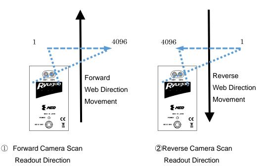
Figure 4-10-2-1 Correlation of Camera Scan Readout Direction and Object
