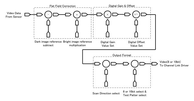
Figure 4-3-1 FPGA Processing Block Diagram
