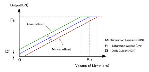
Figure 4-9-1 Saturation Exposure and Dark Current Output
