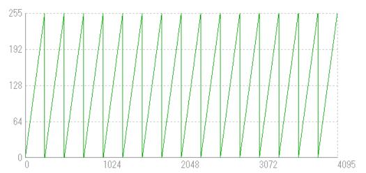
Figure 4-10-4-1 Waveforms of the horizontal ramp pattern on Mono8
