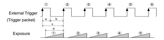
Figure 4-7-2-1 External Trigger (Timed) Exposure Mode
