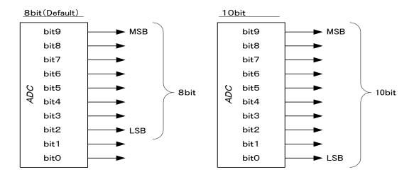
Figure 4-10-1-1 Assignments of Digital Data
