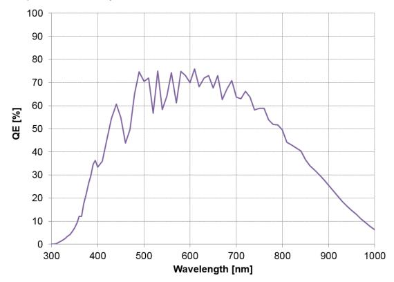
Figure 1-4-2 Quantum Efficiency
