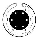
Figure 3-3-1 Power Supply Connector (HIROSE: HR10G-7R-6PB)
