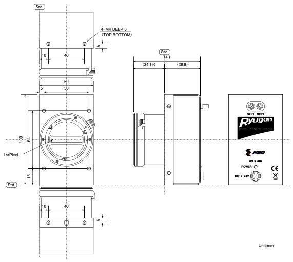
Figure 2-3-1 Dimensions of the Camera (F Mount)
