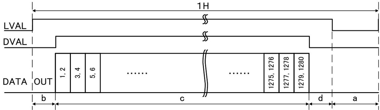
$a=62\text{CLK}$ ,  $b=36\text{CLK}$ ,  $c=640\text{CLK}$ ,  $d=46\text{CLK}$ ,  $1\text{H}=784\text{CLK}$ ,  $1\text{CLK}=50\text{MHz}$
