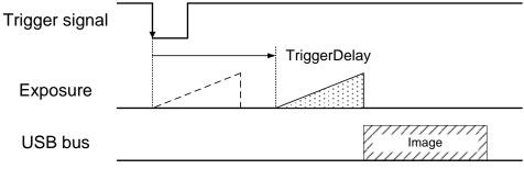
Fig. Trigger Delay
