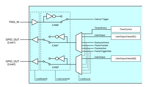
Fig. GPIO internal circuit diagram
