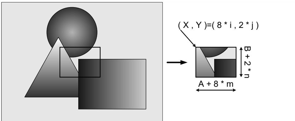
In the scalable mode, camera reads out only necessary area at the normal speed and reads out other area at high speed. The trigger interval can be shorter when the vertical height size is small.
