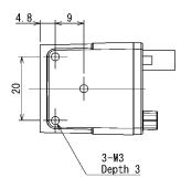
Specification Main material : Aluminum die-cast metal Processing : Cation coating (black)
