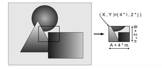
In the scalable mode, camera reads out only necessary area at the normal speed and reads out other area at high speed. The trigger interval can be shorter when the vertical height size is small.
