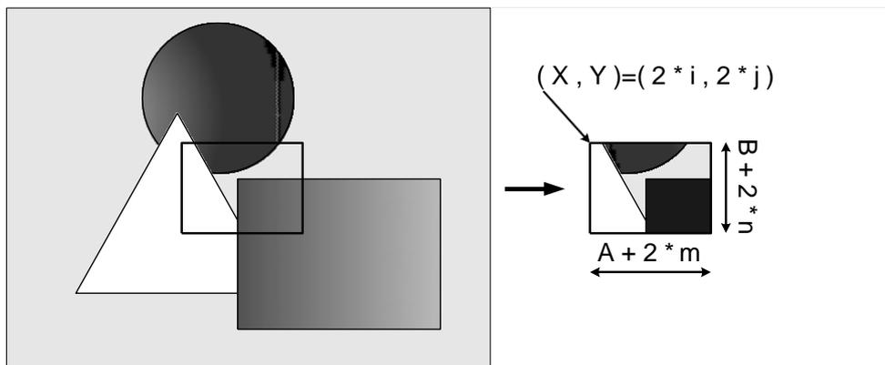
In the scalable mode, camera reads out only necessary area at the normal speed and reads out other area at high speed. The trigger interval can be shorter when the vertical height size is small. However, the trigger interval cannot be shorter when the horizontal width size is small, due to the operation mechanism of the CCD sensor.
